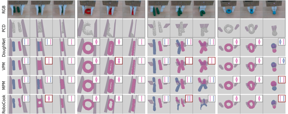
Fig. 6: Qualitative Comparison on Real Sequences. Full-sequence predictions from an initial partial observation. Results are shown at time steps t = \{5, 10, 15\} . Erroneous topology predictions (white boxes, top right) feature a dark red border.
