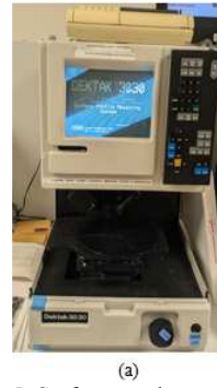
Fig. 5: Surface roughness measurement setup (a) Dektak 3030 profilometer (b) Profilometer tip used for surface roughness measurement of a sample
