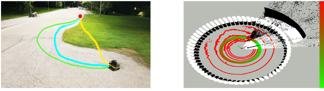
Fig. 6: First real-world experiment: G-Nav can not avoid mud; G-Nav(yellow), V-Nav(green), VG-Nav(cyan). K_{nav} = 0.5 .
