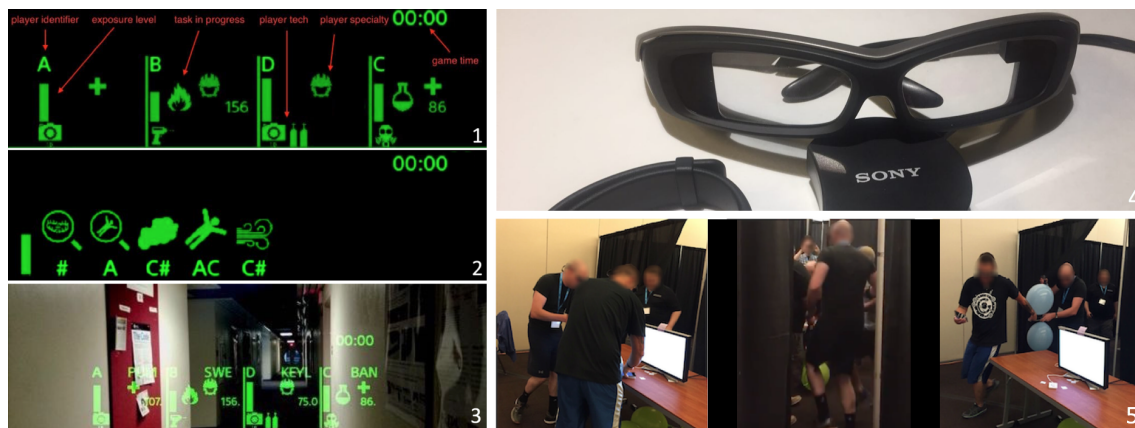
Figure 2. The designed wearable interfaces for the disaster response mixed reality live action role playing game ( Icehouse ). 1. The team status view with player information. 2. The decision support view shows the optimal order of activities to clear a room, as well as which player should do what. 3. The interface is displayed on top of the transparent lens of the smart glasses. 4. The Sony SmartEyeglass used in the game. 5. Photos of the live mixed reality game.
