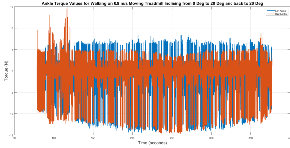
Fig. 5. Plot of left and right ankle torque values for hardware experiment on the Cassie bipedal robot walking on an inclined moving treadmill moving at a constant speed of 0.9 m/s. The treadmill is gradually inclined from 0 degrees to its maximum incline of 20 degrees and back to 0 degrees.
