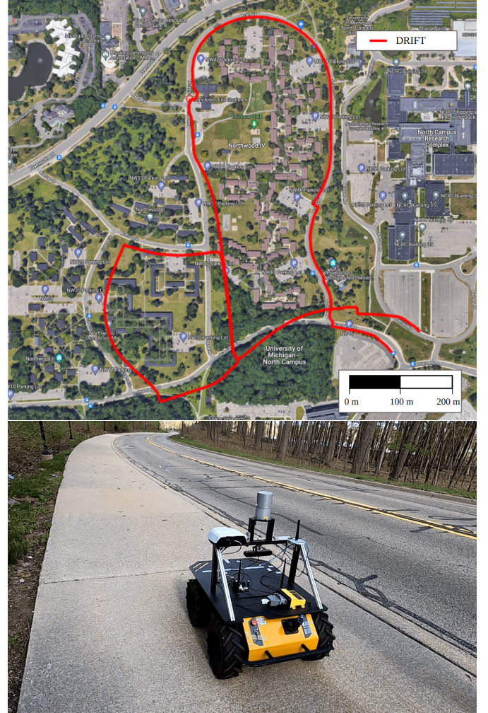
Fig. 1. Estimated trajectory from DRIFT overlapped with the satellite image at the University of Michigan North Campus. A Clearpath Robotics Husky robot was driven on the sidewalk for 55 minutes, with a total path of around 3 kilometers. Consuming proprioceptive measurements only, DRIFT can produce highly accurate estimations for long-horizon operations. This experiment demonstrates the potential of DRIFT to be a reliable odometry system in perceptually degraded situations.
