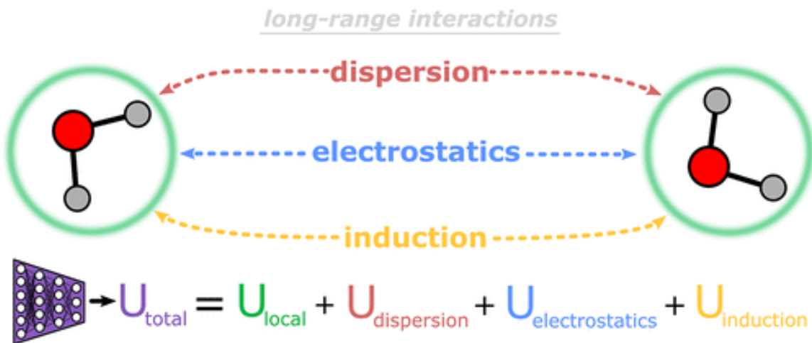
Figure 8. Summary of the general energetic contributions composing the total potential energy ( U_{\text{total}} ) of a system. U_{\text{local}} refers to the short-range system energies and is typically inferred using a machine learning model trained on local features. Dispersion corrections, electrostatics, and induction are collectively referred to as the long-range interaction energy contributions. Adapted with permission from Ref. [142].
