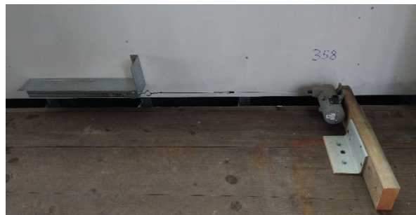
Figure 5: String potentiometer used to measure subassembly slip relative to the building
