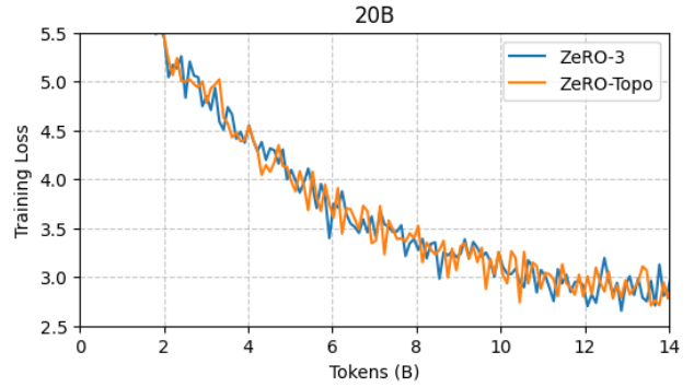
Fig. 10. Loss curve for ZeRO-Topo vs ZeRO-3 with GPT-NeoX-20B
