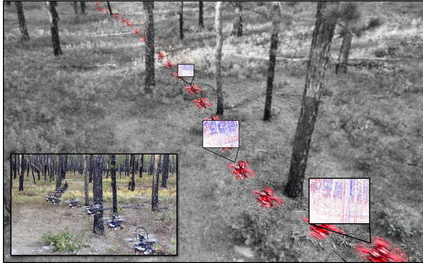
Figure 1: Our event camera-equipped quadrotor avoids static obstacles under considerable ego-motion. Our simulation pre-trained, events-to-control policy is fine-tuned with real-world perception data, such as that from a forest. Red lines indicate avoidance maneuvers during the flight. We demonstrate obstacle avoidance in indoor, outdoor, and dark environments.
