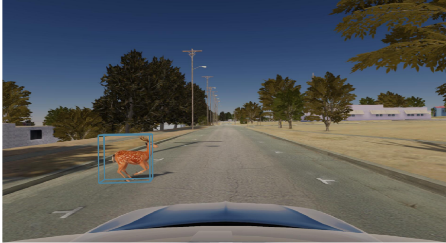
Figure 17: Camera Image for the scenario in Fig. 15. Blue bounding box is the ground truth detection. The camera fails to detect the deer crossing the road (misdetection failure).
