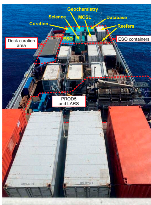
Figure F1. MMA Valour deck plan, Expedition 389. ESO containers (red) at the aft of the vessel included mobile containers for curation, multisensor core logging, geochemistry, database, and network management; two refrigerated core reefers; the ESO office; and the Science office. Here, the reefer of core from the first leg has been lifted off. For the starboard core curation area, coverings were required to mitigate the impact of direct sunlight on the core and provide adequate protection from weather.
