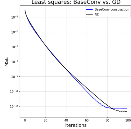
Figure 4: BASECONV can express high-precision gradient descent: our implementation of the weight construction reaches 10^{-13} MSE in practice.
