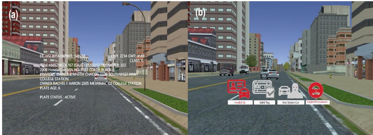
Figure 2: Adaptive AR-HUD MCT display showing a) Regular MCT information for low workload; and b) Simplified MCT information for high workload with low clutter.
