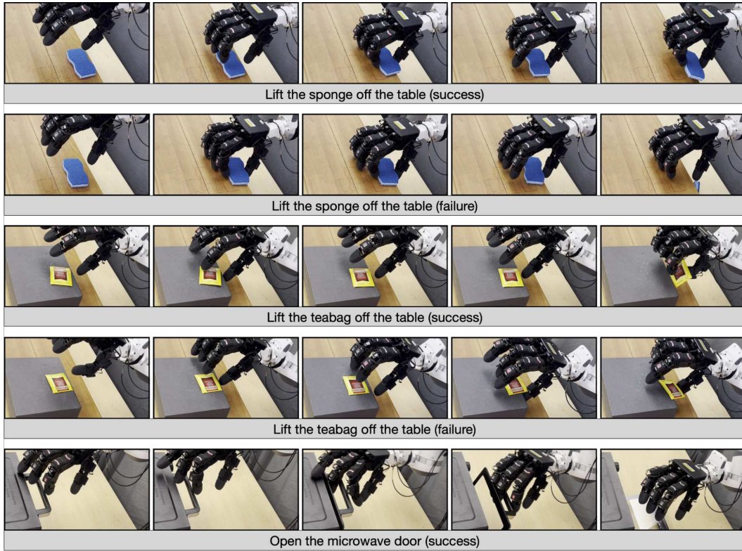
Figure 6: Rollouts on Allegro Manipulation with our DynaMo-pretrained encoder.
