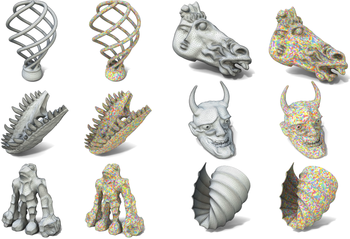
Fig. 12. Anisotropic triangular meshes and their corresponding anisotropic RVD results of our NASM on some complicated surfaces from Thingi10k dataset.
