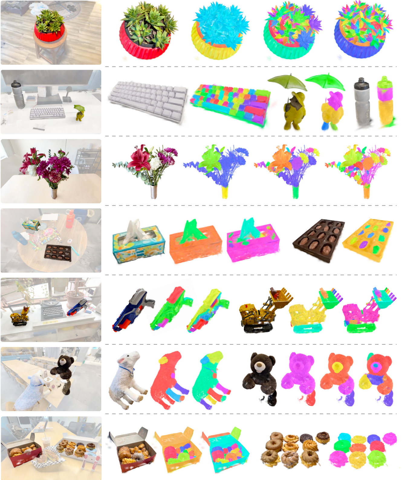
Figure 7. Results: From a GARField we extract objects from the global scene by selecting top-level clusters, then visualize their local clusters at decreasing scales. GARField can produce complete 3D object masks, and break these objects into meaningful subparts based on the input masks. We use Gaussian Splats [12] to produce these visualizations in 3D. See the website for video results.
