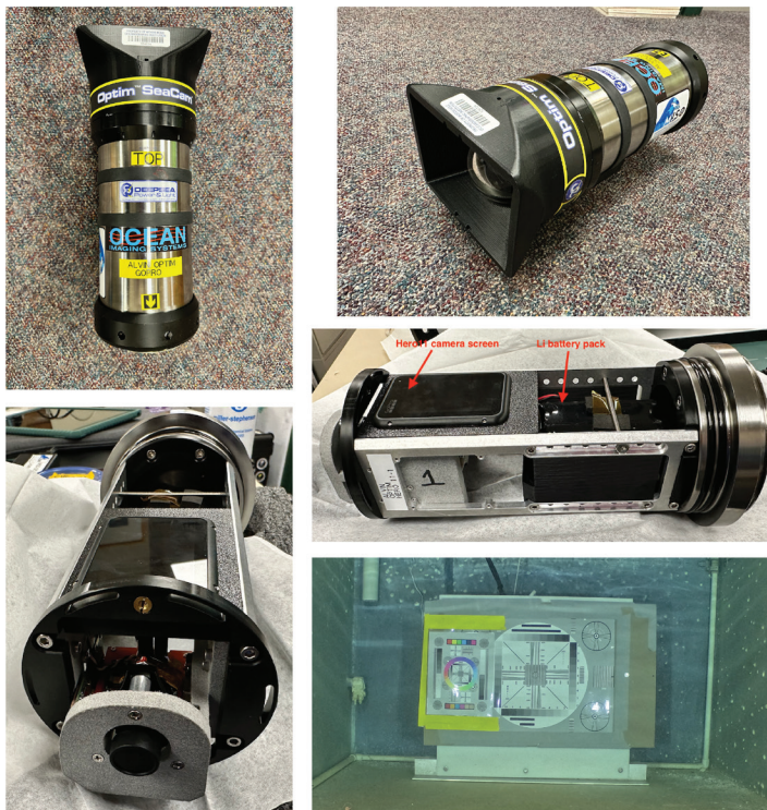
Figure 12: 11 km-rated DeepSea Optim SeaCam camera housing for Alvin 's GoPro HERO11™ still and video camera system resulting from the collaboration between DeepSea, EPO-OIS, Back-Bone, and the WHOI-MISO Facility. The three-element high pressure corrected dome port optic (two lens elements plus the dome) is the same design as the one used in the DeepSea Digi SeaCam and Super SeaCam housings (see Figures 3-5).
