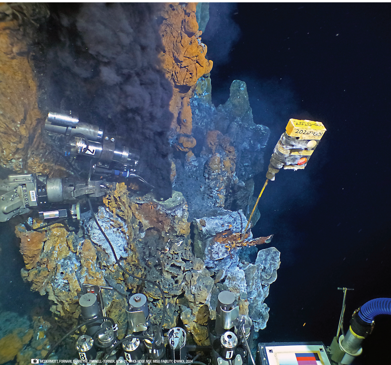
Figure 20: 27MP image of hydrothermal fluid sampling at “Nick’s” vent during Dive 5235 at the YBW-Sentry hydrothermal vent ~700 m east of the axis of the East Pacific Rise near 9° 54’N in February 2024. Image was shot using a 3rd generation MISO Digi SeaCam system using a GoPro HERO11™ camera on Alvin ’s “brow” (above pilot’s viewport). Instrument to the right of the vent orifice is a EPO-MISO high-temperature vent fluid logger [21] that was imbedded in the chimney top that was broken off the structure to allow the fluid sample to be collected.
