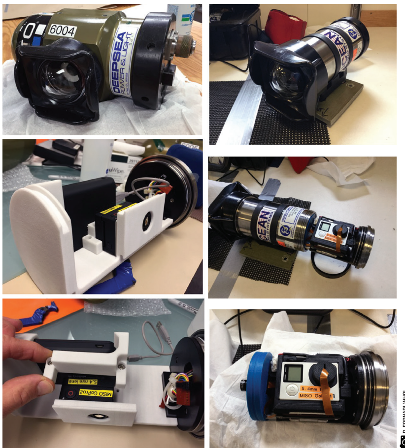
Figure 3: MISO GoPro™ camera systems, 1st and 2nd generation cameras that use GoPro HERO4™ imaging modules. Left panel shows the 1st generation system in the DeepSea Digi SeaCam housing and right panel shows the 2nd generation cameras in the DeepSea Super SeaCam housing, both rated to 6,000 m operating depths.
