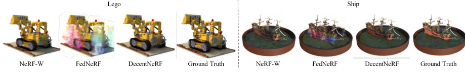
Fig. 5: Qualitative results on Novel Blender dataset: DecentNeRF simultaneously removes unwanted personal content (‘lego persons’) while reconstructing fine details of global content (‘lego excavator’ and ‘ship’). In contrast, FedNeRF [13] hallucinates ‘blobs’ where personal content exists in user views.
