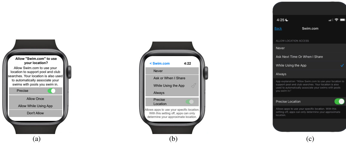
Figure 9: Illustration of permission model on iOS-watchOS. (a) The user grants permission on the watch. (b) The watch setting is disabled against any permission decision change. (c) The user can modify permission settings via the phone setting.
