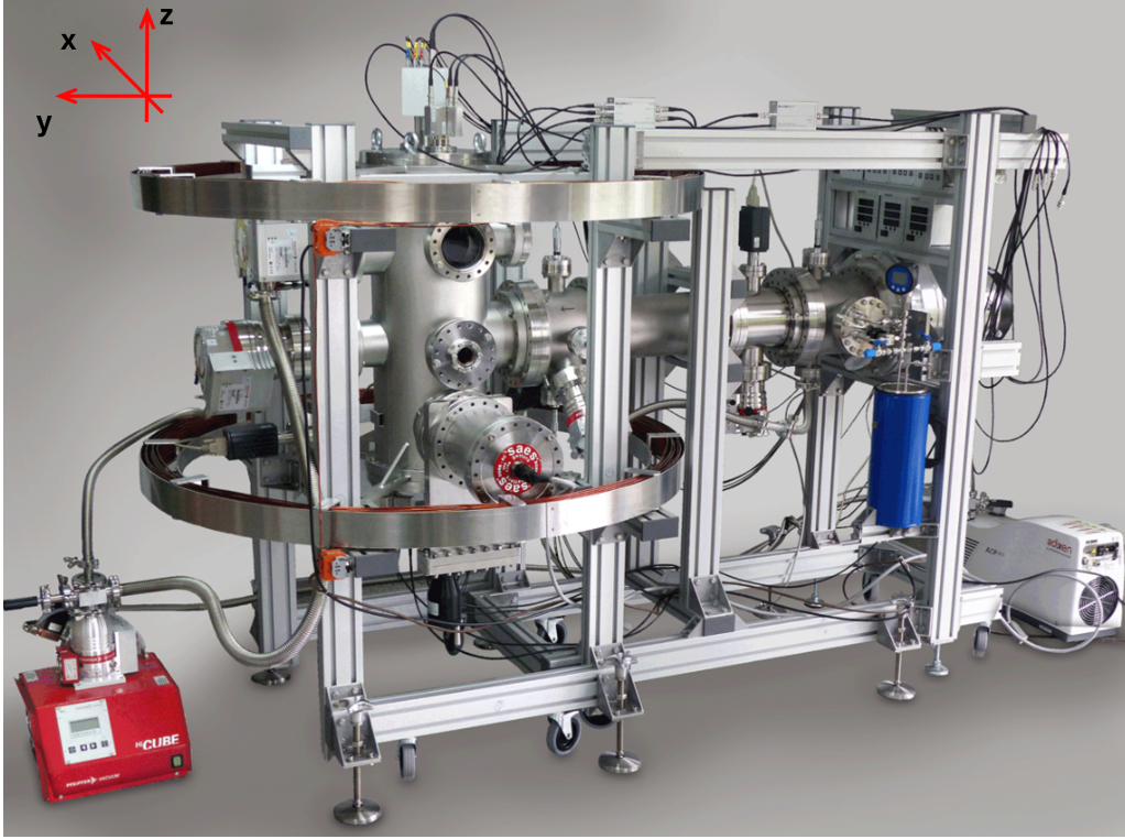
Figure 2.2: COLTRIMS setup showing the main chamber with the spectrometer and electronics. The gas jet enters the interaction region along the y -axis, the laser beam enters the chamber through a window along the x -axis, and the spectrometer is fixed along the z -axis. Figure is adapted from [59]
