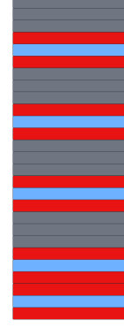
Figure 3: 10-sided hammering example. There are 5 aggressor pairs (red) where each pair is sandwiching a victim row (blue).
