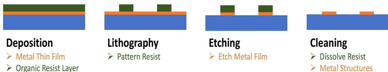
Figure 1.2 Schematic of conventional “top-down” method involving; sputtering of metal layer and deposition of a masking resist, lithographically removing portions of the resist layer to form a pattern, etching away the unmasked metal layer, and cleaning off the remaining resist to reveal the patterned metal features underneath.
