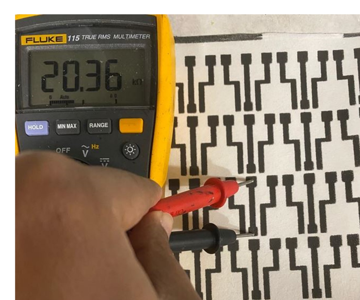
Figure 2: 3D printed conductive sensors from Graphene on 10% LMPLA nonwoven mat.
