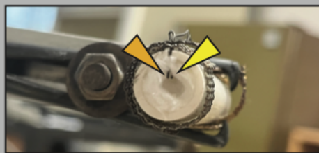
Fig. 1a: Sample holder and thermocouples with vesiculated sample protruding from end. Colors correspond to T-t graphs, below.
