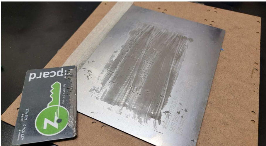
Fig. 31. Solder Stencil with applied solder paste.
