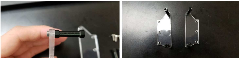
Fig. 120. Acrylic pieces with M3 standoffs attached.
