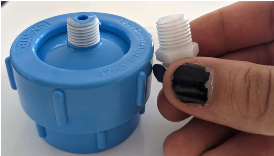
Fig. 22. Threading with Teflon tape applied.
