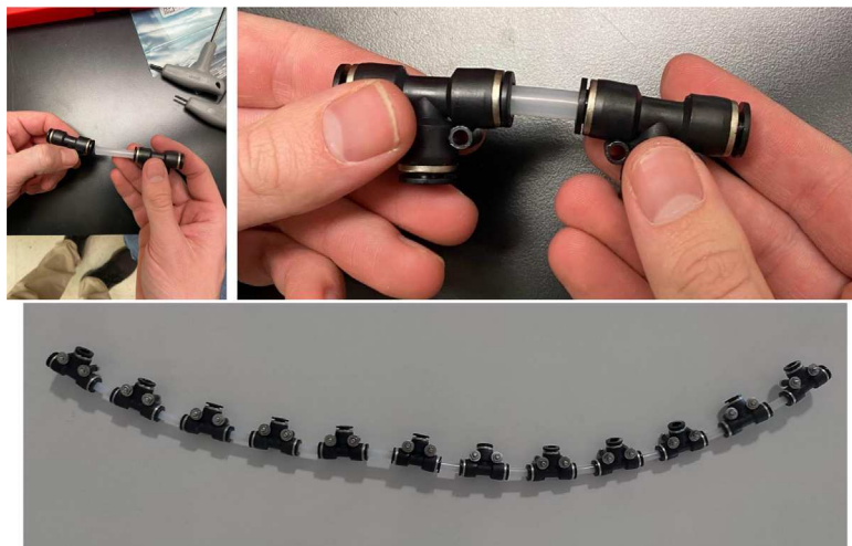
Fig. 76. The bottom hydraulic push to connect tee sub-assemblies.
