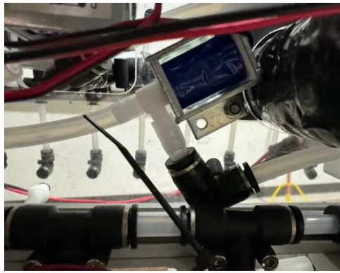
Fig. 104. The air valve mounted to the sampler.
