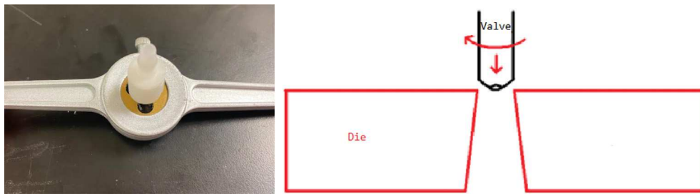
Fig. 15. Process for threading the opposite side of the spring check valve.
