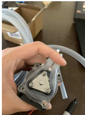
Fig. 96. Pump tubing inserted into pump.
