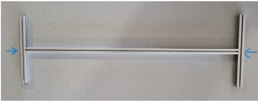
Fig. 64. The 200 mm and 610 mm extrusion top frame sub-assembly.
