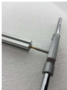
Fig. 52. Tapping the extrusion pieces with the M3 tap at entire thread length.
