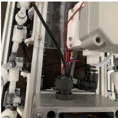
Fig. 164. The central component wires inserted into cable gland.
