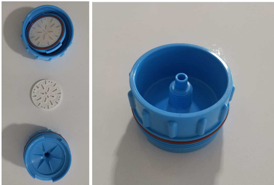
Fig. 17. Disassembled Advantec filter housing.
