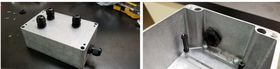
Fig. 122. The cable glands attached to the electronics box.
