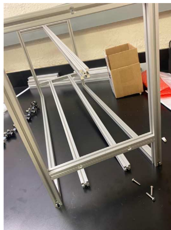
Fig. 85. The sampler frame with bottom extrusion bolts removed.
