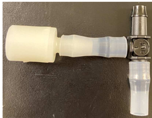
Fig. 45. The Cut check valve attached to the barbed tee.
