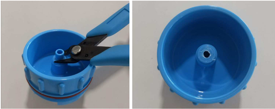
Fig. 18. Removing filter housing extruded tube.
