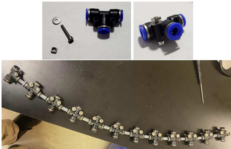
Fig. 73. The bolts, washers, and square nuts inserted into The-push to connect cross sub-assembly.
