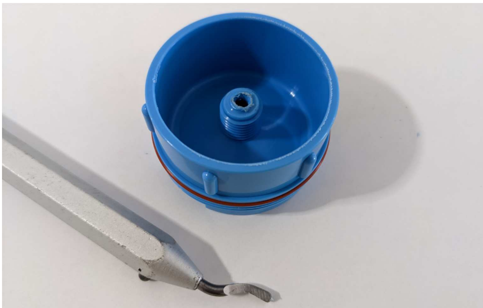
Fig. 19. Deburring the modified filter housing.
