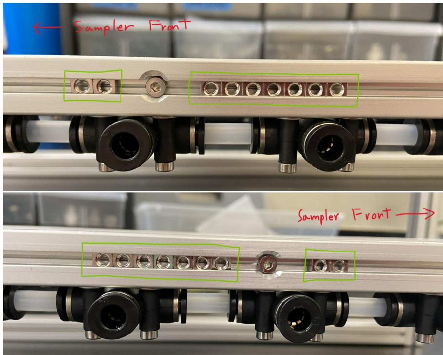
Fig. 90. The final square nuts applied to the sampler frame.
