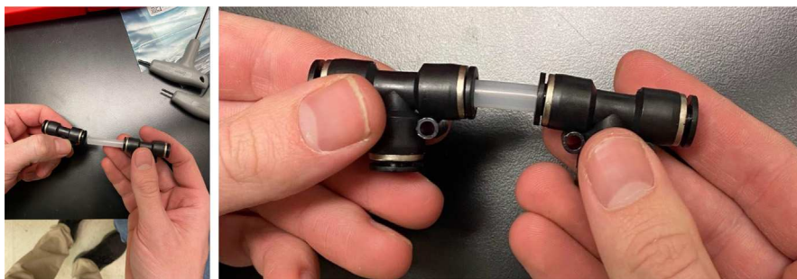
Fig. 72. The top hydraulics push to connect cross sub-assembly.
