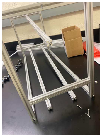
Fig. 80. The sampler frame with bottom extrusion bolts removed.
