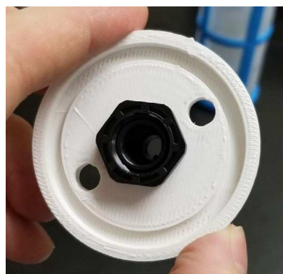
Fig. 132. The PG7 glad mounted to the 3D printed lid.
