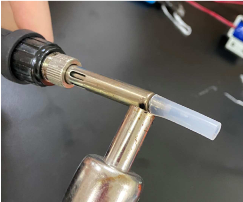
Fig. 41. Thick-walled tubing being heated until flexible.
