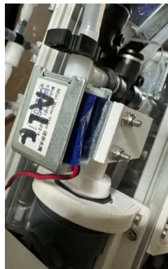
Fig. 106. The alcohol valve mounted to the L-bracket.
