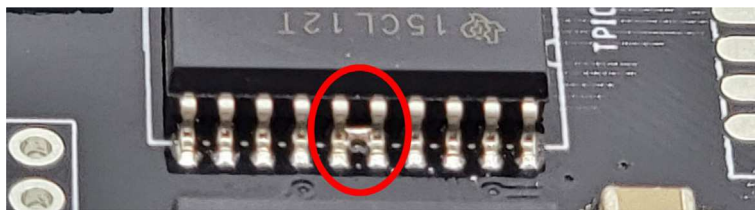
Fig. 37. IC component displaying solder bridging.
