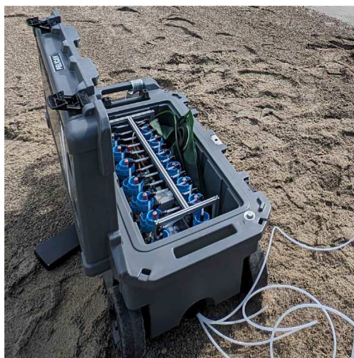
Fig. 9. The sampler deployed in a pelican case for weather protection.
