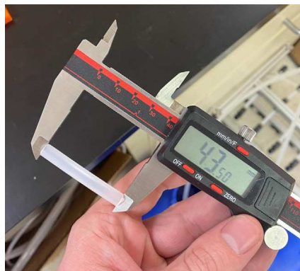
Fig. 75. The Caliper measurements for hydraulic thin-walled tubing.
