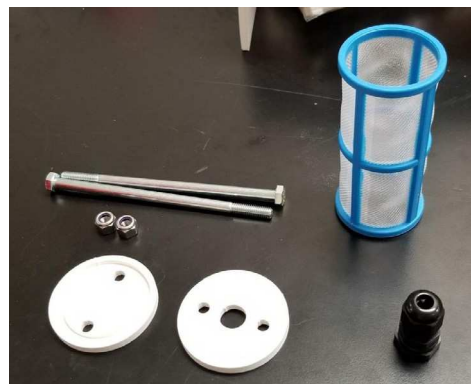
Fig. 131. The pre-filter sub-assembly components.
