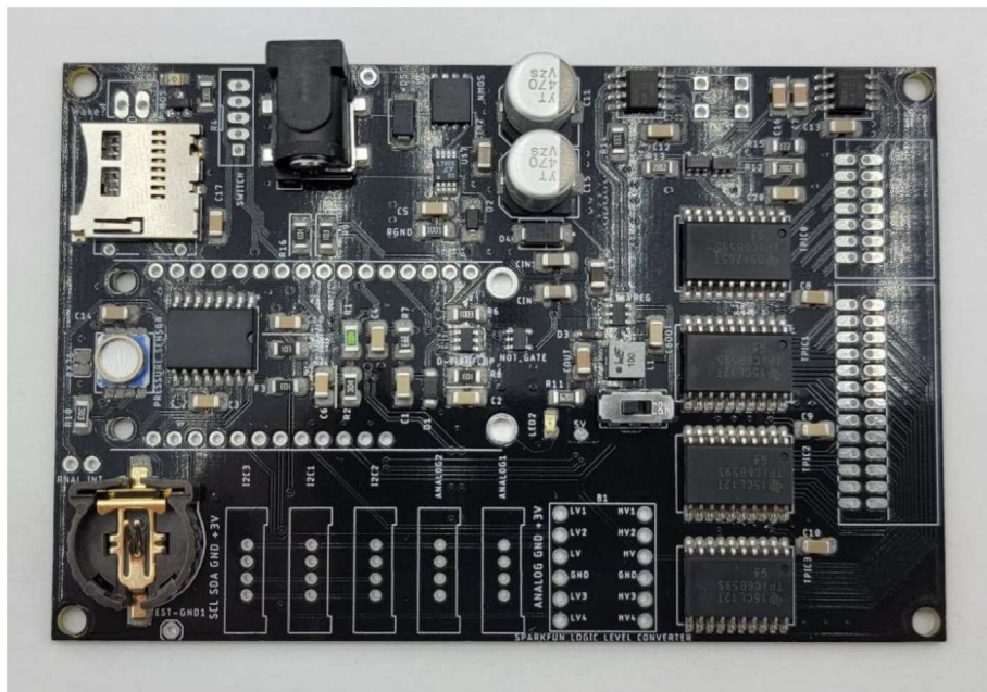
Fig. 33. Filled PCB with SMD components applied to solder paste on board.
