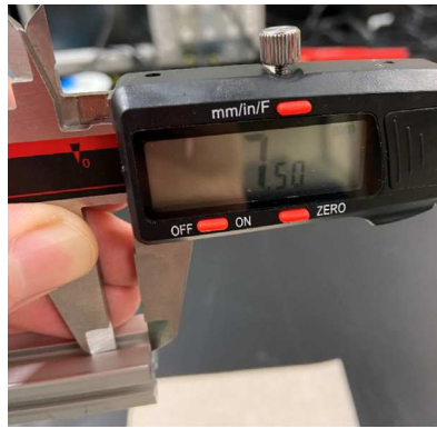
Fig. 57. Caliper used with extrusion to determine hole locations.
