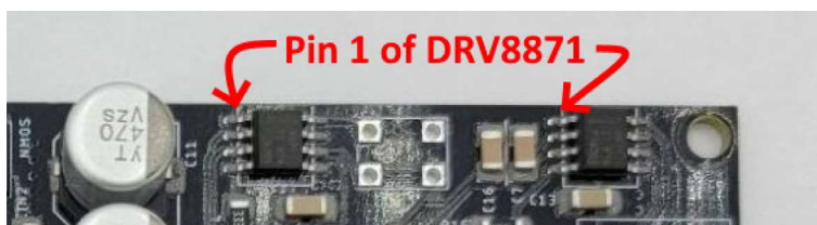
Fig. 34. DV887 Pin 1 location with missing orientation designation.
