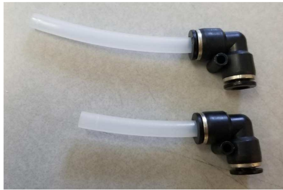
Fig. 74. The top hydraulic 60 mm and 80 mm push to connect corner sub-assemblies.
