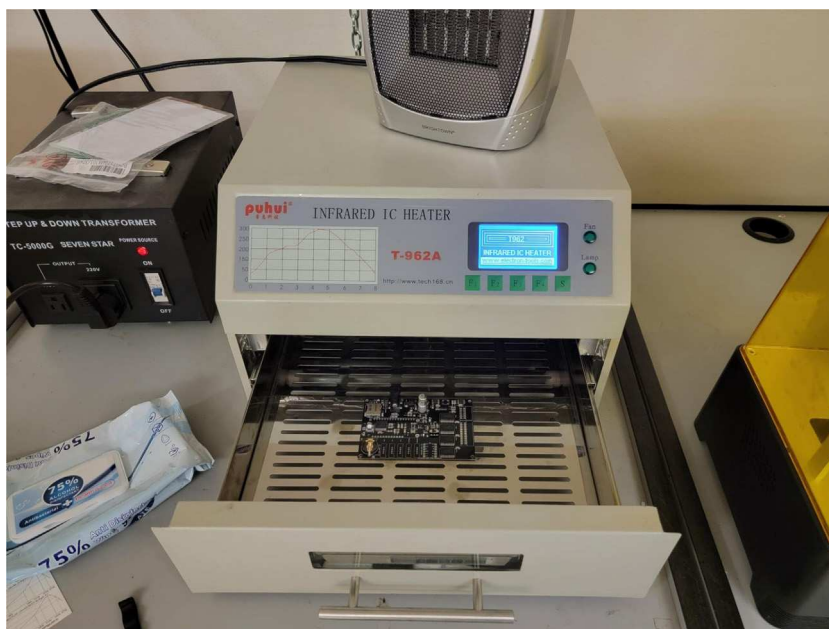
Fig. 35. SMD oven with set components.
