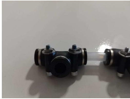
Fig. 77. The M3 bolt, washers, and square nuts applied to the bottom hydraulic push to connect tee sub-assemblies.
