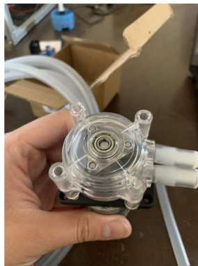
Fig. 97. Closed-pump with barbed tubing.
