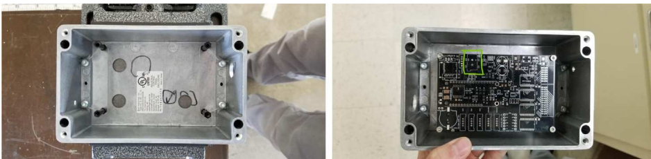
Fig. 121. The self-threading screws mounting the acrylic stand and electronics board.
