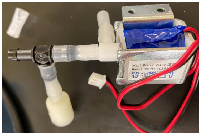
Fig. 46. Barbed tee assembly connected to solenoid valve.
