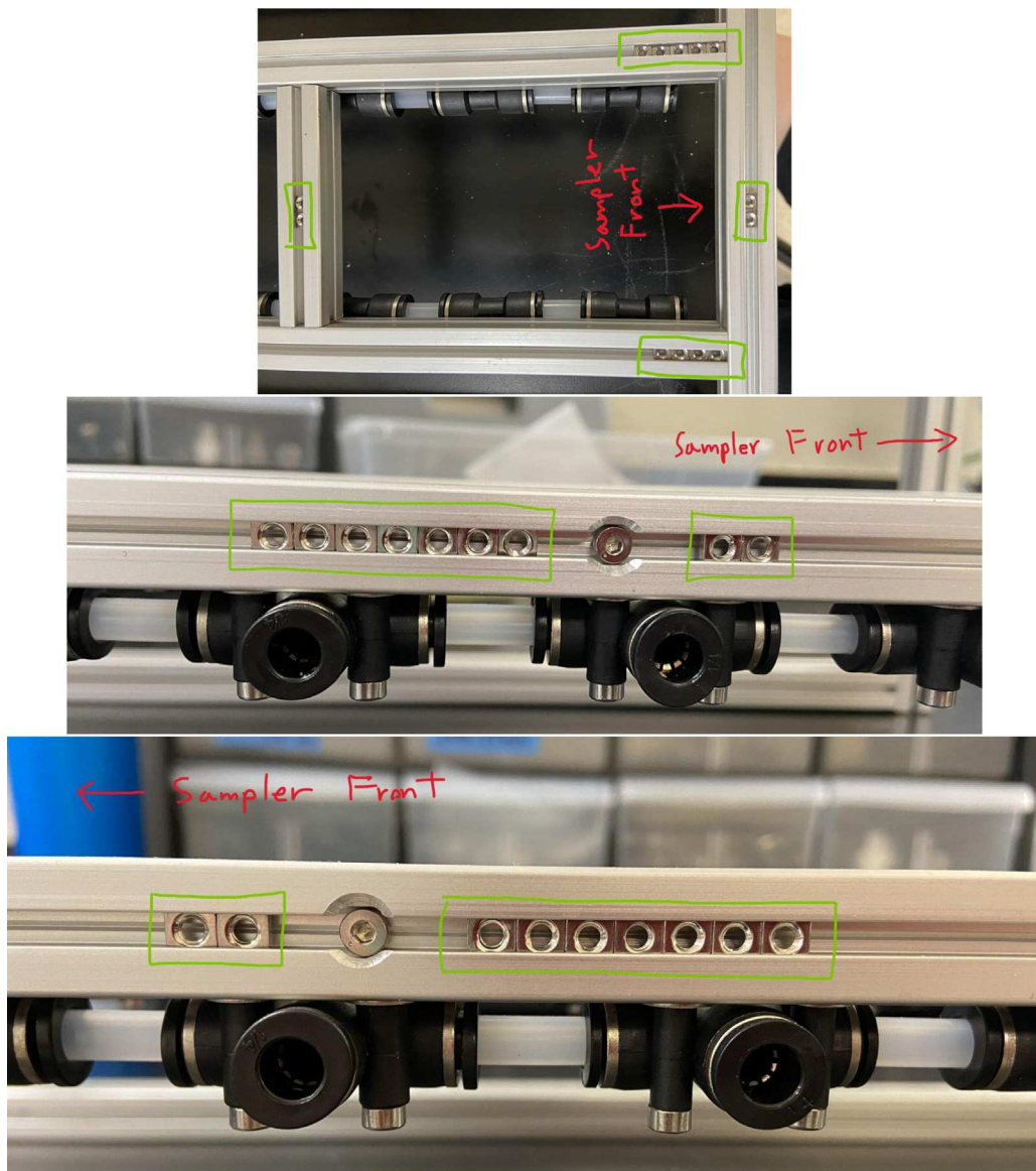
Fig. 89. Square nuts applied to the top, and left of sampler frame.
