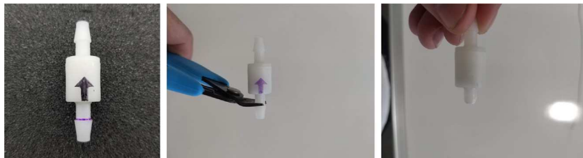
Fig. 13. Process for cutting the barbed tip of the spring check valve.
