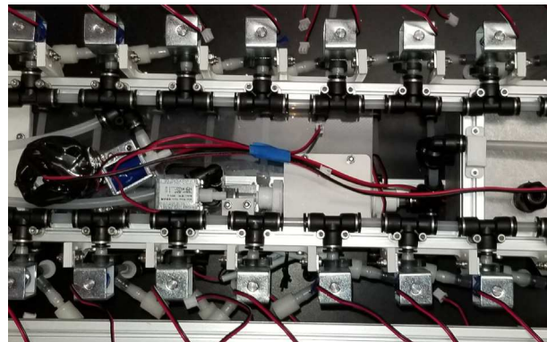
Fig. 135. The pump, air, and purge valve wires separated.
