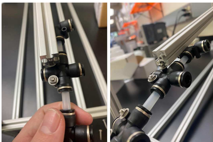
Fig. 81. The top hydraulics inserted into the upper sampler frame.
