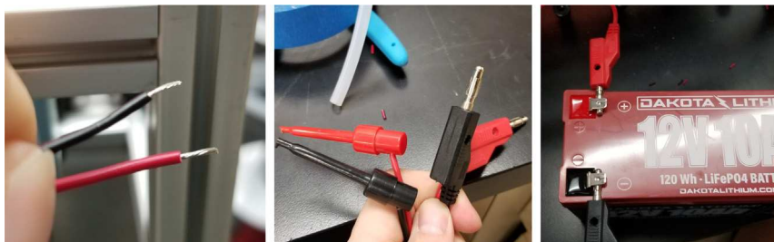
Fig. 137. The stripped wires powered by the battery and alligator clips.
