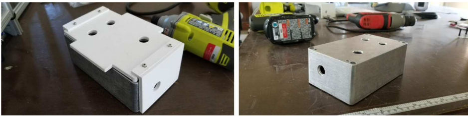
Fig. 118. Electronics box holes cut using the 3D printed Jig.
