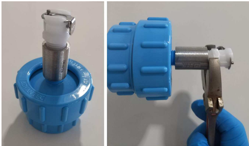
Fig. 24. A modified filter housing with coupling.
