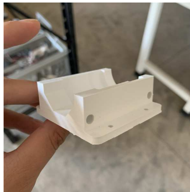
Fig. 100. The ball valve mount with supports removed.
