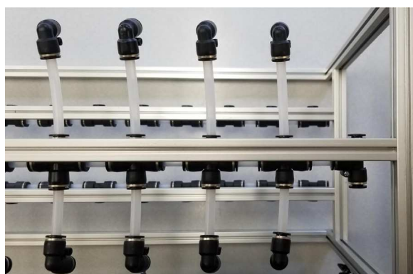
Fig. 83. The corner push to connect sub-assemblies attached to the upper hydraulics.
