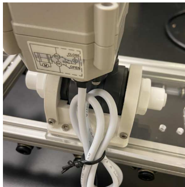
Fig. 103. The ball valve mounted with M3x8 mm bolts.
