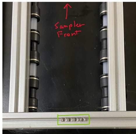
Fig. 79. Square nuts applied to the top sampler frame.
