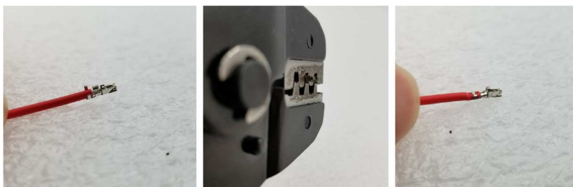
Fig. 157. The crimp secured via crimping tool.
