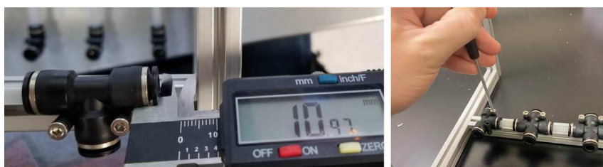
Fig. 82. The upper hydraulics in correct frame position.
