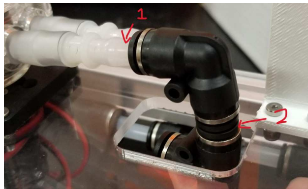
Fig. 108. The pump barb converter connected to push to connect corners.
