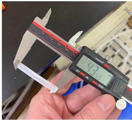
Fig. 71. The Caliper measurements for hydraulic thin-walled tubing.
