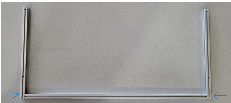
Fig. 66. The 310 mm and 610 mm extrusion side frame sub-assembly.
