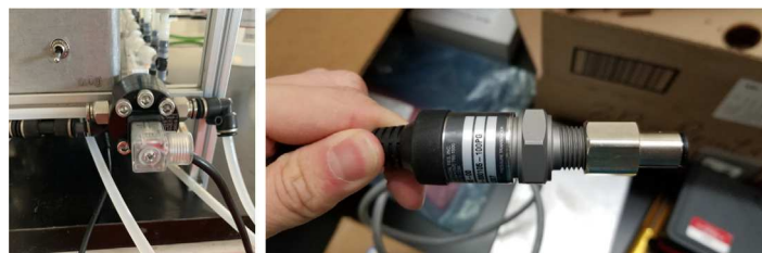
Fig. 172. The pressure sensor with required fittings.
