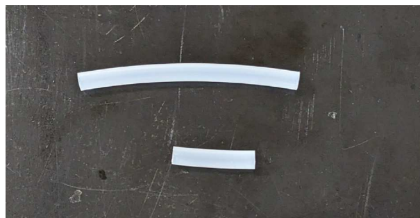
Fig. 12. 28 mm and 77 mm length thin-wall tubing.
