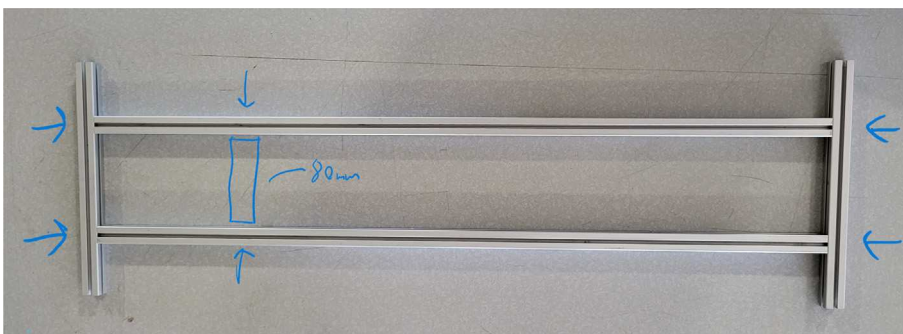
Fig. 62. 610 mm and 200 mm assembly with location of 80 mm extrusion.
