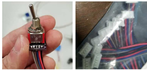
Fig. 168. The DPDT switch and PCB connector.
