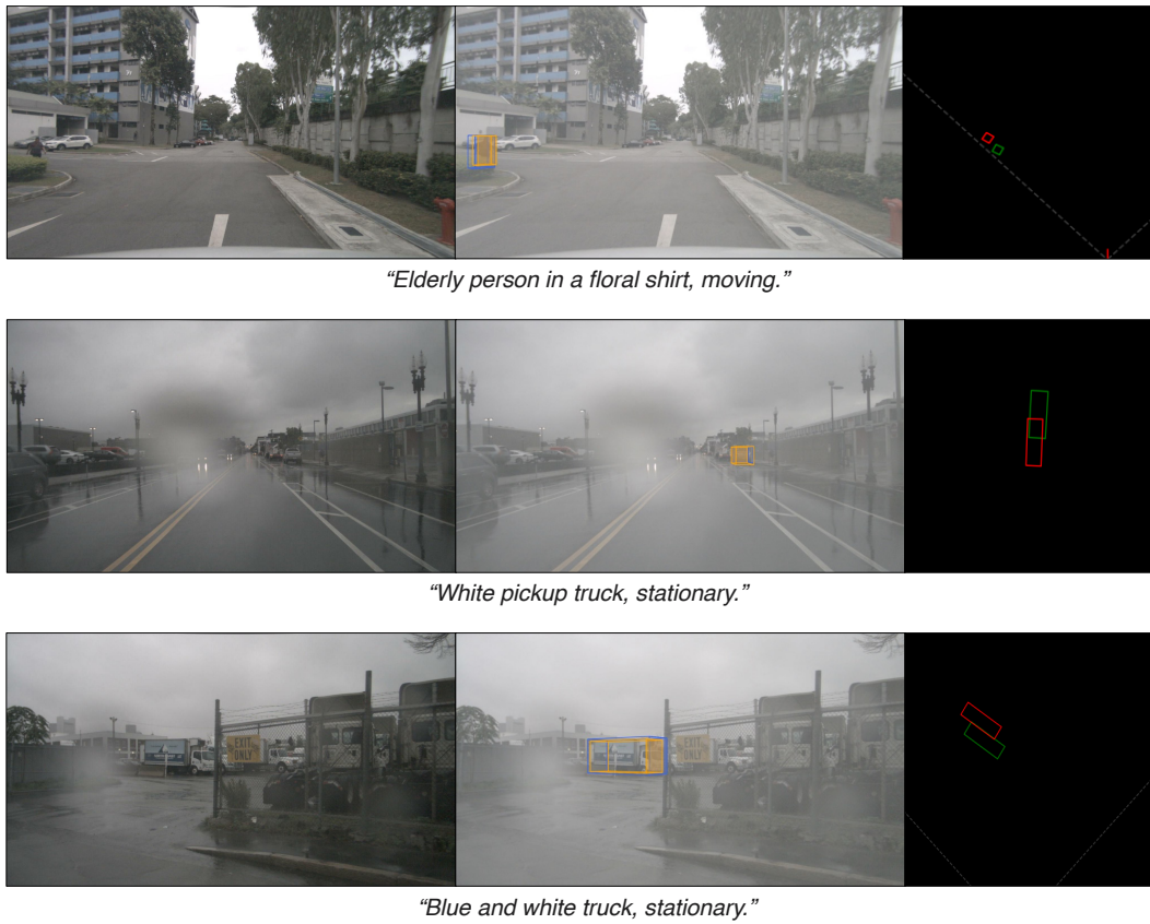
Figure 18: Failure cases of DriveLM-Grounding images. The error mainly attributes to incorrect depth. Each row has the original image (left), projected 3D box prediction and ground truth (middle), and BEV image (right). Blue box is the ground truth and Orange box is the prediction. In BEV images, Green box is the ground truth and red box is the prediction.
