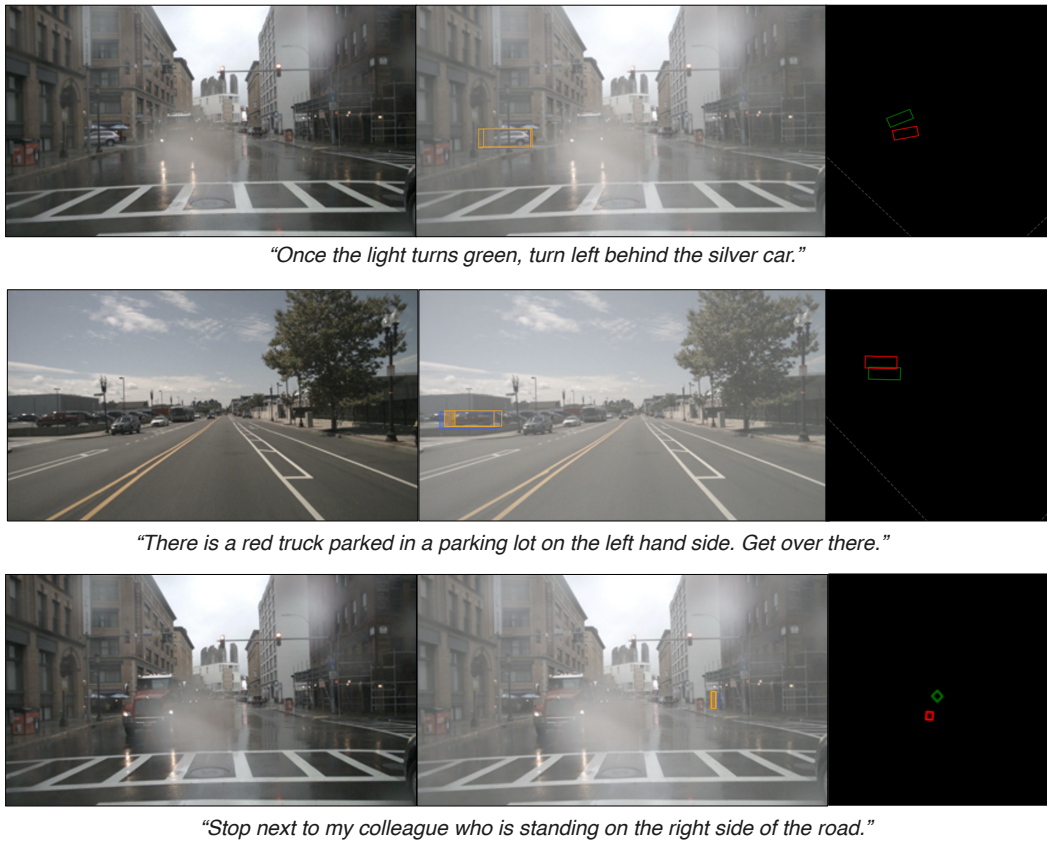
Figure 20: Failure cases of Talk2Car images. The error mainly attributes to incorrect depth. Each row has the original image (left), projected 3D box prediction and ground truth (middle), and BEV image (right). Blue box is the ground truth and Orange box is the prediction. In BEV images, Green box is the ground truth and red box is the prediction.
