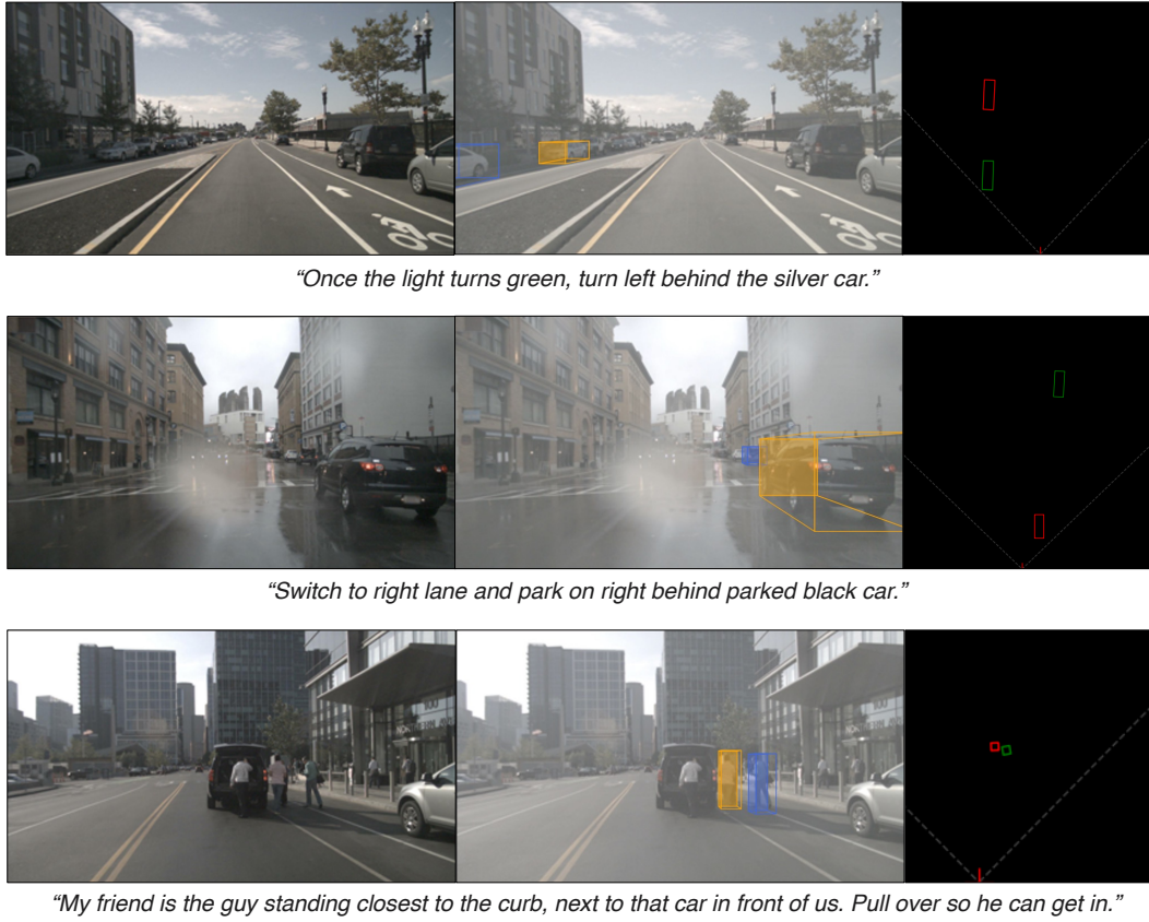
Figure 21: Failure cases of Talk2Car images. The error mainly attributes to semantic mismatch. Each row has the original image (left), projected 3D box prediction and ground truth (middle), and BEV image (right). Blue box is the ground truth and Orange box is the prediction. In BEV images, Green box is the ground truth and red box is the prediction.
