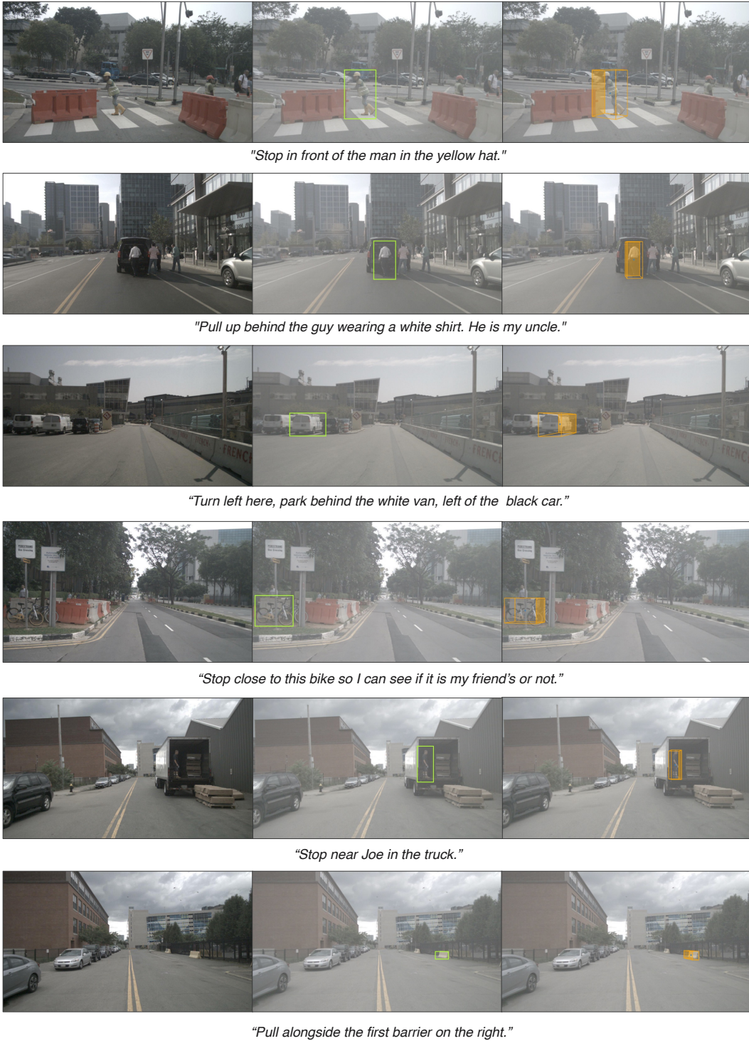
Figure 9: CUBE-LLM visual chain-of-thought prompting inference. The first column is an input image, the second column is the 2D bounding box prediction, and the third column is the final 3D bounding box prediction prompted with the 2D prediction and text.
