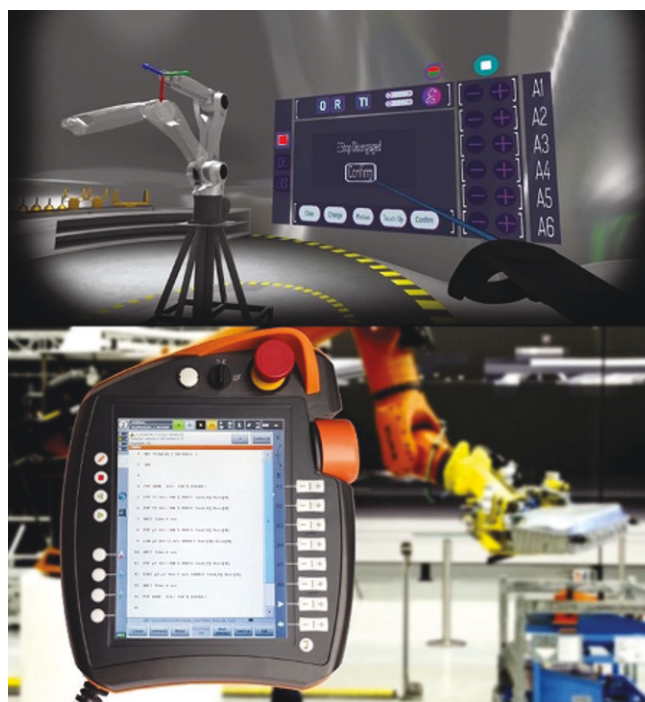
Figure 2. Scene from the VR learning prototype demonstrating how the command panel corresponds to a physical teach pendant in real world.
