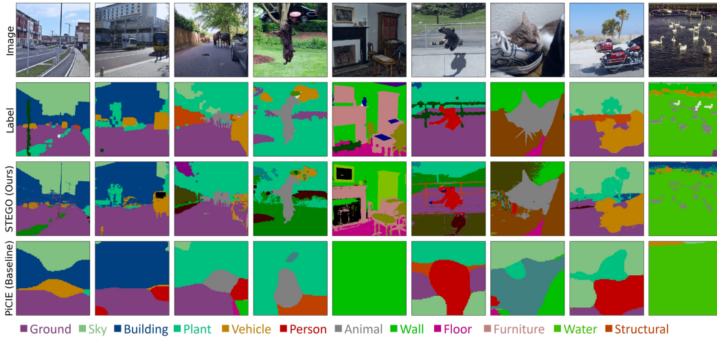
Figure 1: Unsupervised semantic segmentation predictions on the CocoStuff (Caesar et al., 2018) 27 class segmentation challenge. Our method, STEGO, does not use labels to discover and segment consistent objects. Unlike the prior state of the art, PiCIE (Cho et al., 2021), STEGO’s predictions are consistent, detailed, and do not omit key objects.
