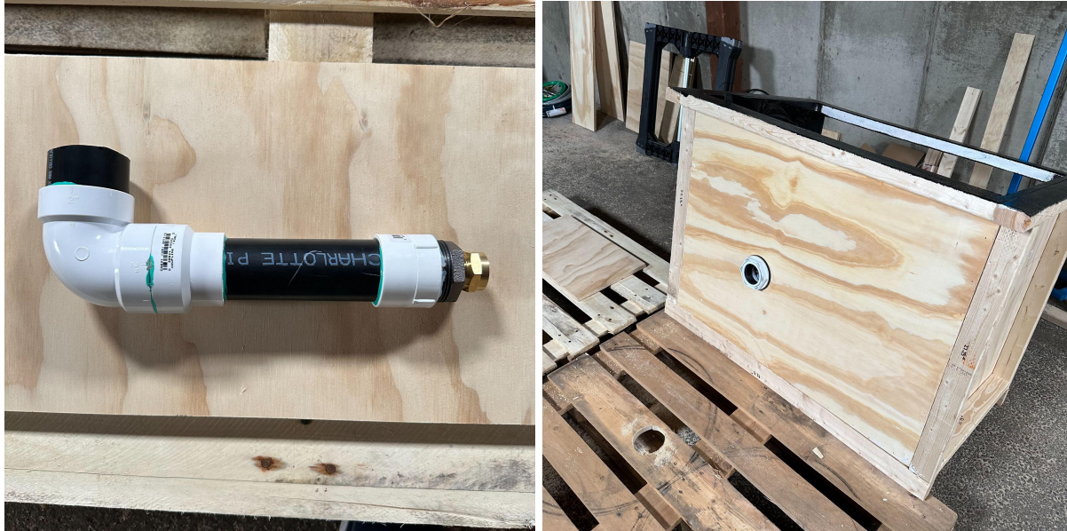
FIGURE 4 Right-angle Pipe underneath Box 1. The tub drain transitions from 2 in (5.08 cm) diameter pipe, to 1.5 in (3.81 cm) diameter pipe, down to a metal hose connection.
