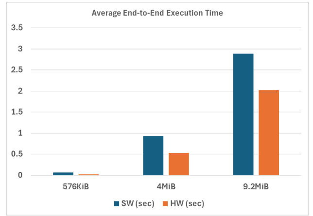
Fig. 5: End-to-End program execution time, including kernel and data transfer times, measured in seconds.
