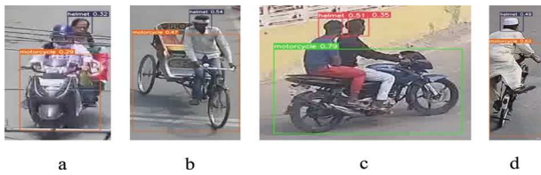
Fig. 6. Visualization of failure cases: a) wrongly detected helmet b) wrongly detected helmet and motorcycle c) dark hair detected as helmet and d) cap detected as helmet.
