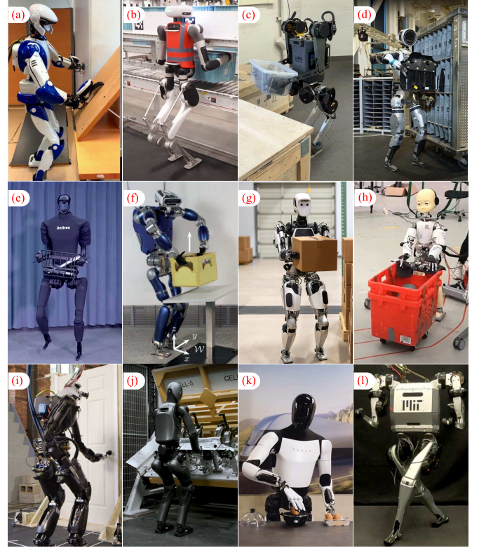
Fig. 1. Humanoids executing locomotion and manipulation tasks: (a) HRP-4 wipes a wood board while adapting to terrain [1]; (b-g) Object pick and place by Digit, Hector [2], Atlas, H1, TORO [3], and Apollo; (h) iCub pushes a cart [4]; (i) Nadia opens a door [5]; (j-k) Object manipulation by Figure 02 and Optimus; (l) MIT humanoid whole-body push recovery [6].
