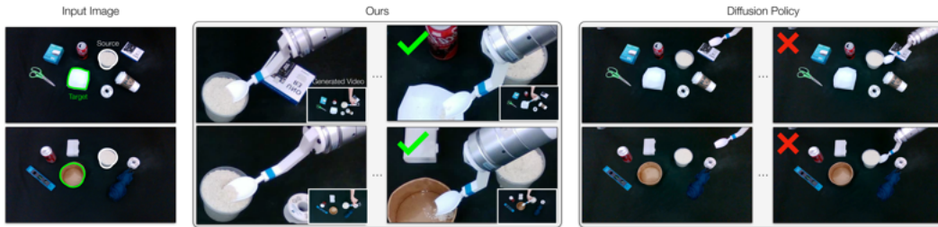
Figure 5: Scooping Qualitative Results. We provide the input image on the left (without the overlays provided for illustration) to our model and Diffusion Policy, and show the output trajectory on the right. Our approach succeeds in most trials, while Diffusion Policy is often distracted by other objects in the scene, placing material in the wrong container and failing to scoop accurately. Generated videos are indicated by ■ ■ ■ ■ .
