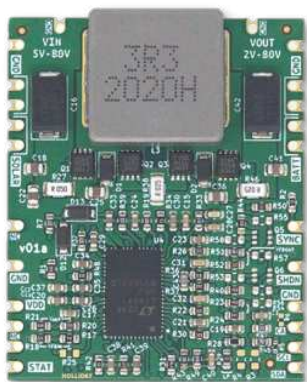
Figure 6: MPPT module based on the Analog Devices LT8491.
