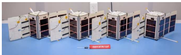
Figure 2: Four 1.5U PY4 spacecraft flight units.
