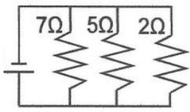
$$\begin{aligned} \frac{1}{R_{eq}} &= \frac{1}{R_1} + \frac{1}{R_2} + \frac{1}{R_3} \\ &= \frac{1}{7} + \frac{1}{5} + \frac{1}{2} = \frac{59}{70} \\ R_{eq} &= \frac{70}{59} = 1.2\Omega \end{aligned}$$
