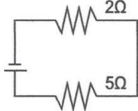
$$\begin{aligned} R_{eq} &= R_1 + R_2 \\ &= 2 + 5 \\ R_{eq} &= 7\Omega \end{aligned}$$
