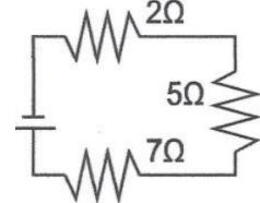
$$\begin{aligned} R_{eq} &= R_1 + R_2 + R_3 \\ &= 2 + 5 + 7 \\ R_{eq} &= 14\Omega \end{aligned}$$
