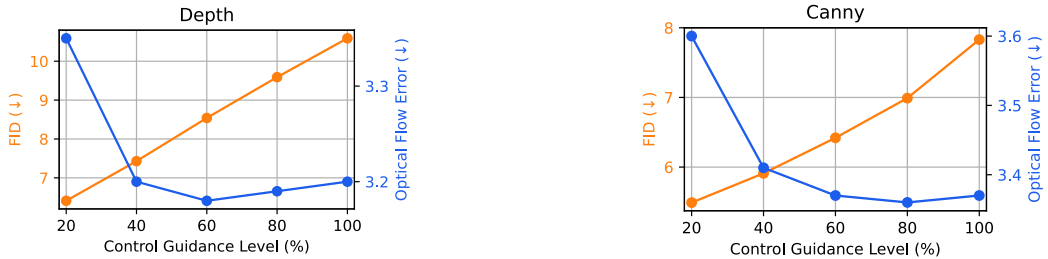
Figure 20: Trade-off between generated visual quality (FID) and spatial control accuracy (Optical Flow Error) on I2VGen-XL . Control guidance level of x represents that we apply CTRL-Adapter in the first x\% of the denoising steps during inference. A control guidance level between 40% and 60% usually achieves the best balance between image quality and spatial control accuracy.
