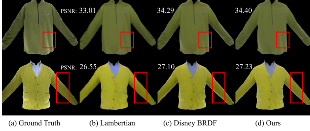
Figure 3. PBR model evaluation. Each mesh is shaded with 3 different shading models and compared with ground truth (a). Notice the sheen around the cardigan sleeve and the wrinkle near the fleece abdomen denoted by the red square. The Lambertian model (b) shows no sheen, Disney BRDF (c) over-estimates the forward scattered sheen, whereas our model (d) produces the best match to ground truth sheen. PSNR values are computed to quantitatively demonstrate the improvement of our model over prior methods.
