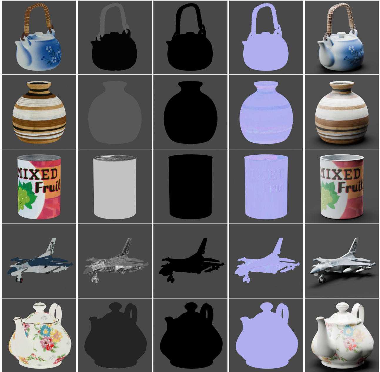
Figure 12. PBR Materials of the example DTC objects (the list of objects in Fig.9 Row 3). From left to right: albedo map, roughness map, metallic map, normal map, and PBR rendering.
