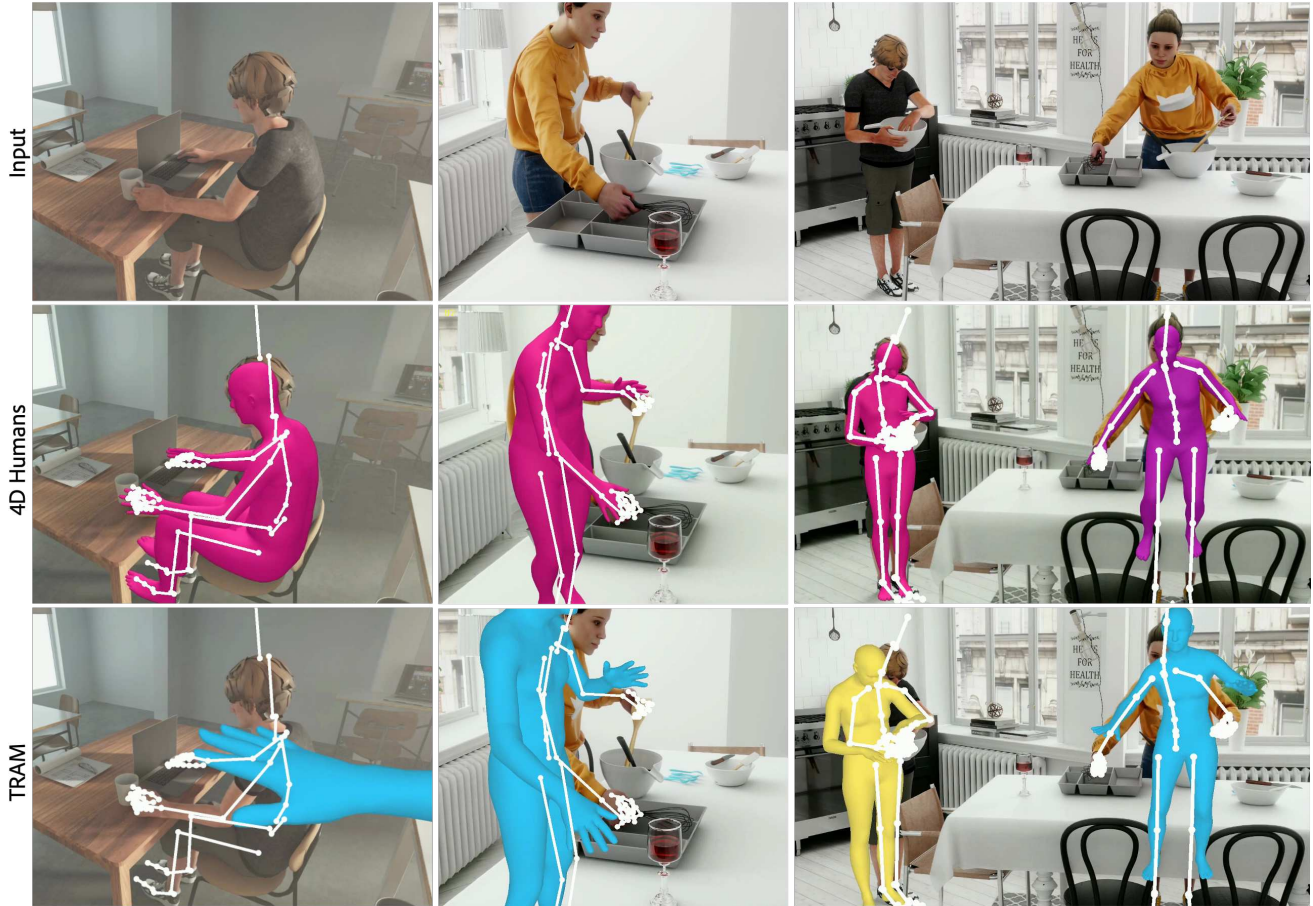
Figure 9. Human motion and pose estimation results on HUMOTO. Comparison between 4D Humans [19] ( Mid ) and TRAM [64] ( Bottom ) on rendered images, showing estimated meshes (colored) against ground truth skeleton (white).
