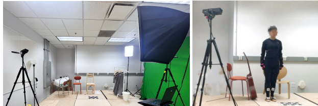
Figure 3. Capture environment. Left: Overview of our capturing environment showing two Kinect cameras, stage, lighting, calibration board, and interaction objects. Right: Calibration procedure with the performer in a standardized position, enabling precise alignment between mocap suit data and camera coordinates.
