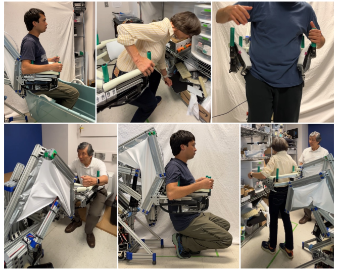
Fig. 9. Six of multiple possible assistance scenarios. Top row: getting into/out of a bathtub, bending down to reach objects, and catching a fall. Bottom row: powered sit-to-stand transition from a toilet, lifting a person from the floor, and walking assistance. Due to IRB restrictions, tasks involving higher risk were tested with an adult.
