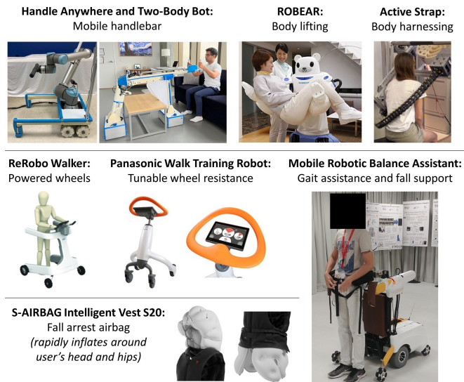
Fig. 1. Examples of eldercare robots, classified by function. From top to bottom row, left to right: body-weight support and/or human body lifting [6] [7] [8] [9], active walkers [10] [11], and fall mitigation [12] [13]. Note that the Mobile Robotic Balance Assistant is able to provide both gait assistance and fall catching, with the caveat of requiring the user to wear a harness.
