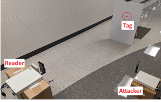
Fig. 3: An example of RFID experiment scenarios.
