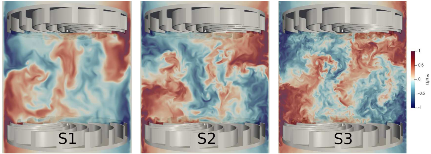
Figure 6.3: Snapshots of configurations S1 through S3 at normalized time ft = \Omega t/2\pi = 3.00 during the isothermal precursor run. As Reynolds number Re_\Omega increases from 4,000 (S1) to 16,000 (S3), finer structures appear whereas the mean velocity field remains largely similar.
