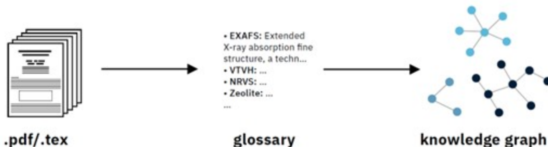
Figure 11: Schematic overview of the GlossaGen project. Textual information is extracted from PDF and LaTeX files and a glossary is generated with terms and their definition. From this, a knowledge graph is created, showing entities and relationships between terms.
