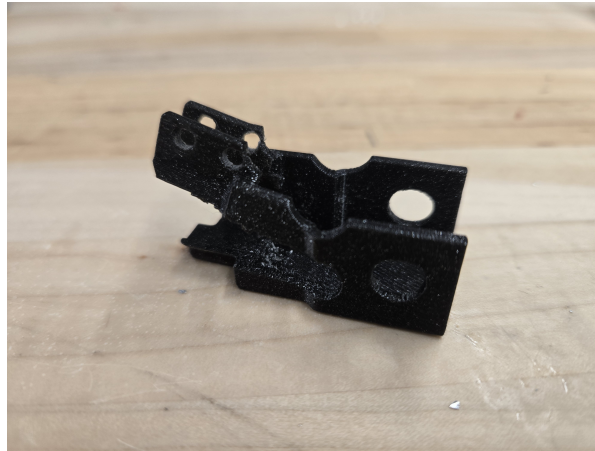
(c) Motor Housing Damage
