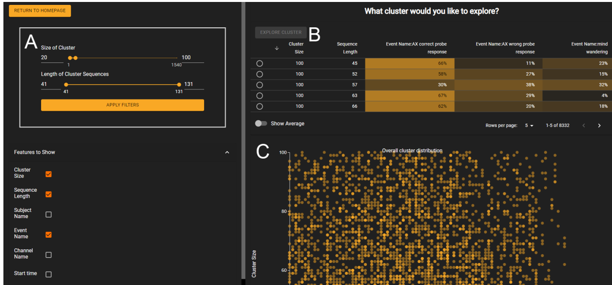
Figure 4.9: Cluster Explorer. BrainEx interface for exploring the clusters consisting of a table of filtering options in the left panel (marked A), a table of the dataset’s clusters and their color-coded feature distributions (marked B), and a visualization showing the overall distribution of clusters in the dataset (marked C). When a cluster is selected, the visualization changes to show that cluster’s representative.
