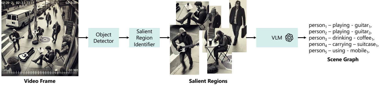
Figure 1. An overview of a VLM-based scene understanding system, which consists of three key steps: (1) object detection, (2) salient region identification, and (3) relationship extraction using a VLM.
