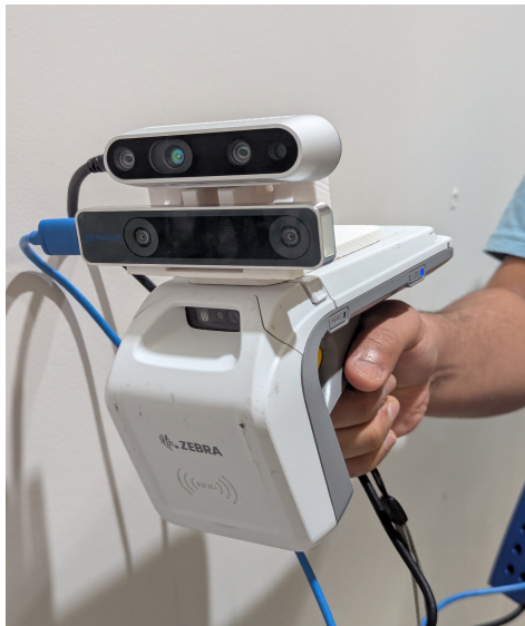
Fig. 5: The RF-visual sensing component: Realsense D435 RGB-D camera (Top), Realsense T265 tracking camera (Middle), and the Zebra RFD8500 Bluetooth Handheld UHF RFID Reader (Bottom).
