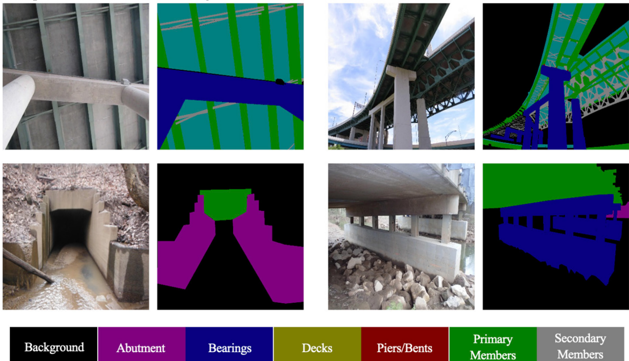
Figure 1. Examples of original images and annotated bridge components.
