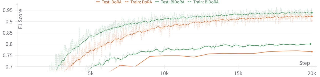
Figure 2: Training and test accuracy versus global training steps on the ModHayes split of the Reuters21578 dataset (Padmanabhan et al., 2016) when fine-tuning a RoBERTa-base model using DoRA and BiDoRA. The training and test curves for DoRA show a larger gap compared to BiDoRA, highlighting the effectiveness of our method in reducing overfitting.
